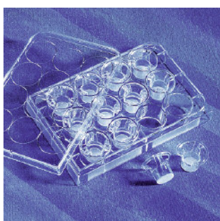
These 12 mm diameter Transwell inserts have a polycarbonate membrane
