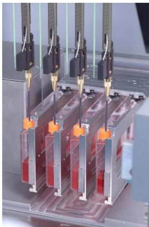
Figure 3-1: Cellerity flask flipper with LiHa tips piercing Corning RoboFlask vessels
